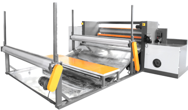
Automatic feeding and receiving device (optional) 自动放料,收料装置可选装
